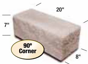
Half Step 7 x 8 x 20 Weight: 84 lbs. Face Area: .39 sq. ft Units per Cube: 24
